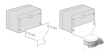
It is recommended to place the top of the unit (where the internal antennas reside), not too close to metallic objects, especially to the mast itself. Ideally the unit should be mounted at the top of the mast. Use tie wraps to fasten the cables to the mast after the mechanical installation is completed.
